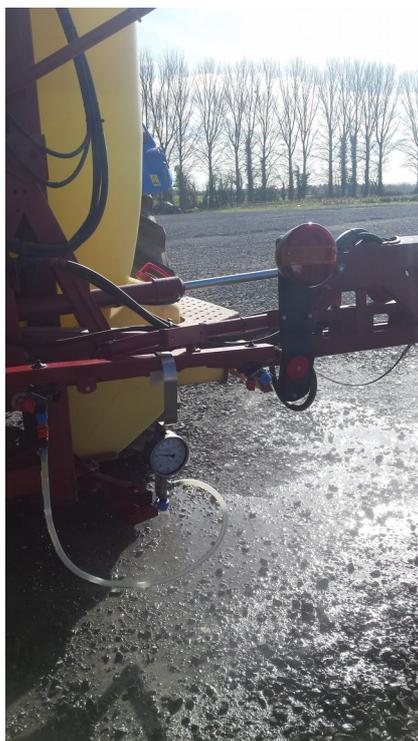
**Nozzle output pressure been tested**
